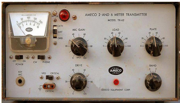
AMECO Model TX-62 was a popular late 1950's phone transmitter for the VHF 6 and 2-Meter bands.
