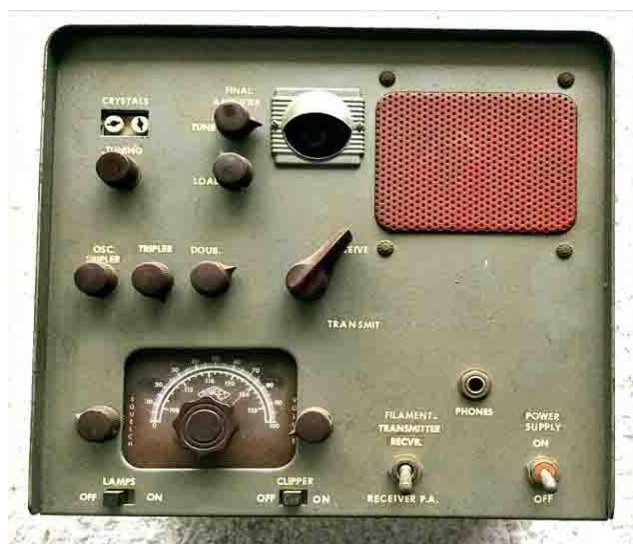
The Gonset Communicator was a series of vacuum tube VHF, AM radio transceivers that were widely sold in the 1950's and early 60's.
