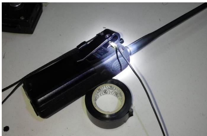
Photo above shows counterpoise wire connected to a screw on the back of the HT
