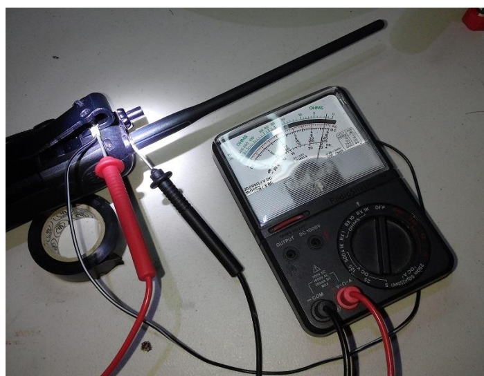
Checking continuity between screw and ground side of antenna. That's all there is to it. 73, K5LUO
