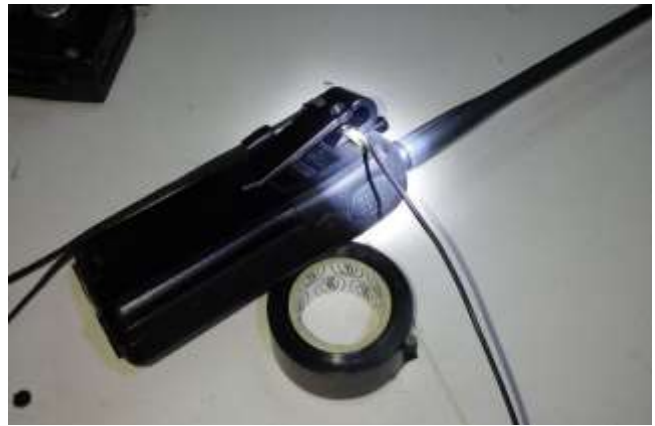
Photo above shows counterpoise wire connected to a screw on the back of the HT.
