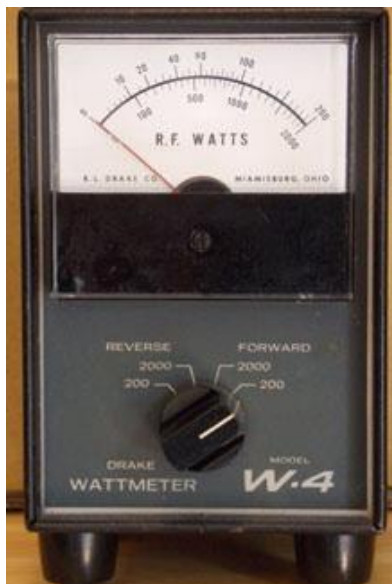
Drake W-4 Wattmeter – scale 200 watts & 2000 watts forward & reverse.
