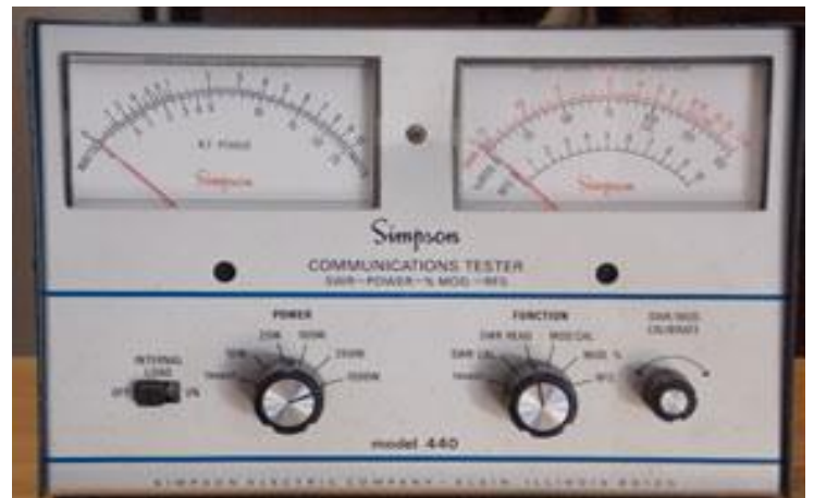
Simpson Mod 440 Communications Tester. Watts, SWR, Modulation %
