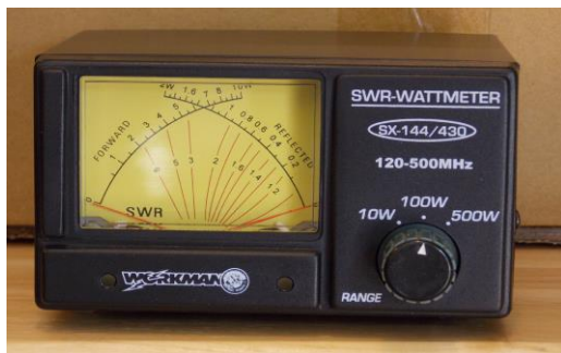
Workman SX144/430 SWR Wattmeter, 12 VDC, 120 MHz – 500 MHz – 10-500 watts.
