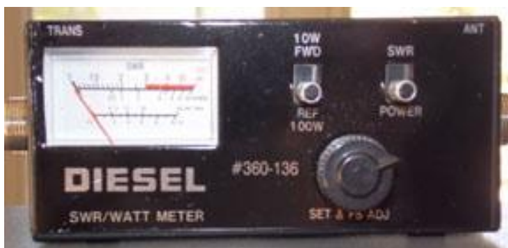
Diesel CB SWR/Watt Meter 10 – 100 Watts
