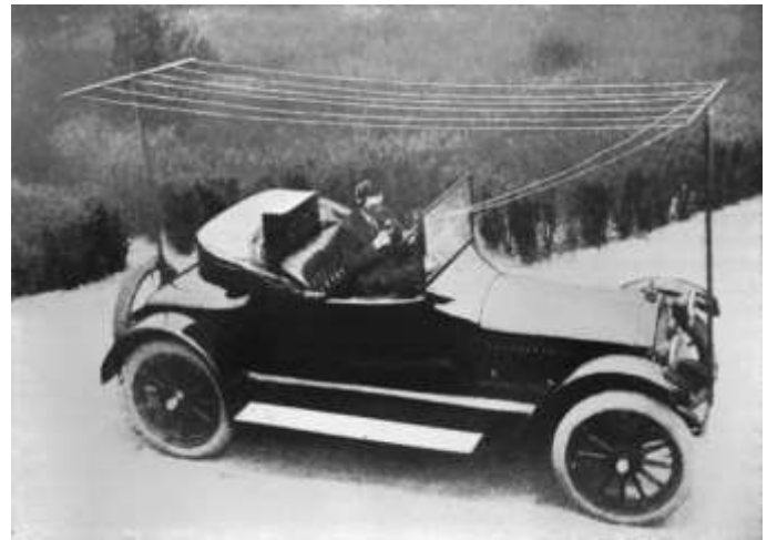
An amateur radio set installed in a car by Alfred H. Grebe, a radio manufacturer of New York in 1919, who is shown speaking into the microphone.
