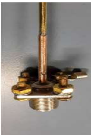
Figure 1. The short copper tube accommodates both the center pin of the SO-239 connector and the brass rod, and solders easily to both. The horizontal radial wires attach at the corners and the coaxial cable connector screws on the bottom
