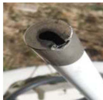
Lighting struck top of cap.
