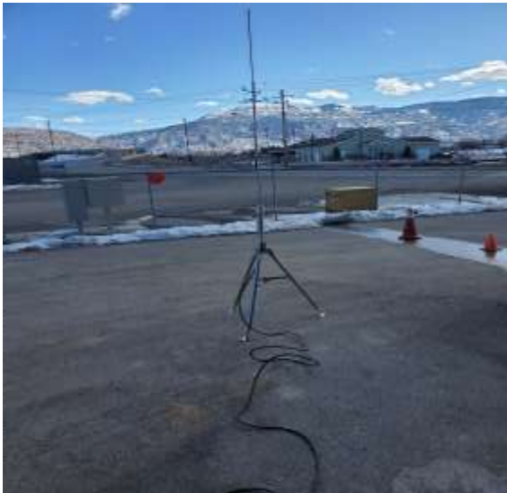
Trying out Dennis (W6DLW) new Wolf River Silver Bullet 1000 Coil HF Antenna. Will be used for 10 Meter contacts.
