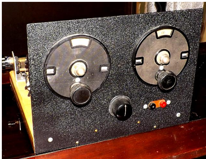
This is an example of an early 1920s style amateur radio receiver that was built from an ARRL Radio Amateur's Handbook article using authentic components of the era.
