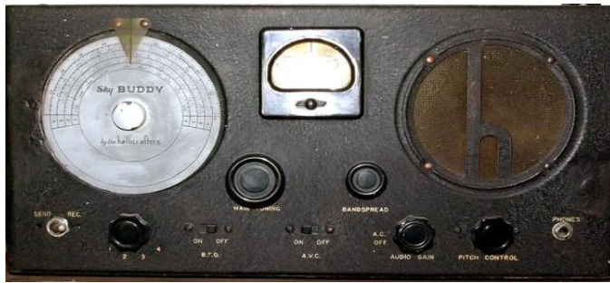
Hallicrafters S-19 "Sky Buddy" was one of the first in a line of hobbyist communications receivers made by the Hallicrafters Company of Chicago, IL.
