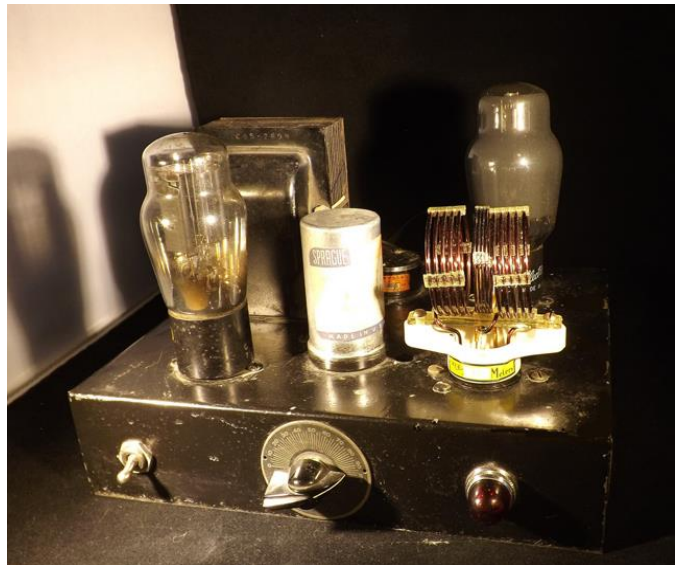
This 1939 vintage 20-Watt CW transmitter, manufactured by the Thordarson Transformer Company, utilizes a 6L6-G as the RF oscillator/RF output tube, along with a Type 80 full-wave rectifier. Following full restoration, the unit was recently placed on the air for a demonstration, and it still kicks out a mean little signal for its size.
