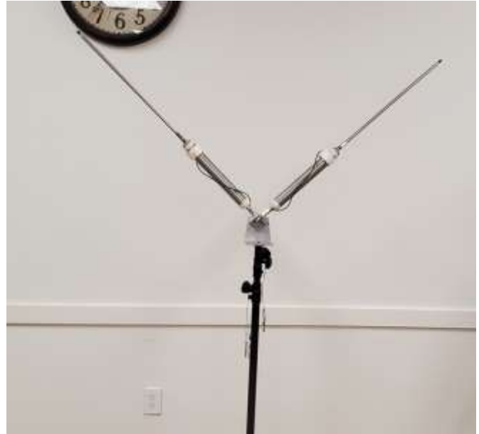
Pictured is the 10-80 M Adjustable Dipole
