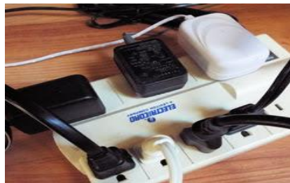
Small household "wall warts" are typically noisy switching power supplies.
